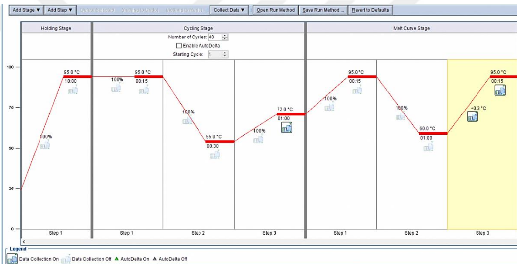
Figure 7. Thermal cycle of real-time PCR reactions.
