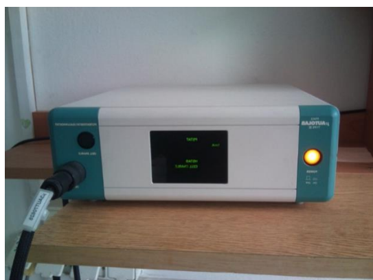
Figure 8. Potentiostat/galvanostat— \mu\text{Autolab GpES} .
