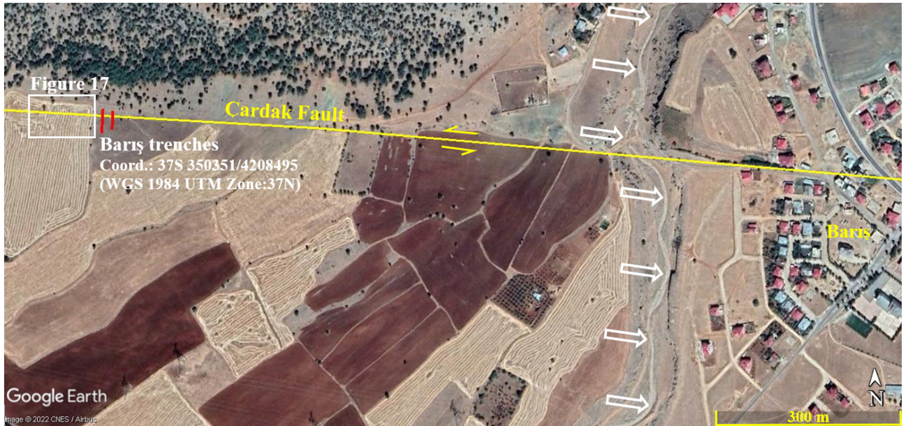
Figure 7. Google Earth image showing the 70-m stream offset through Barış village. White arrows indicate the sinistral deflection emphasized by the stream bed.
