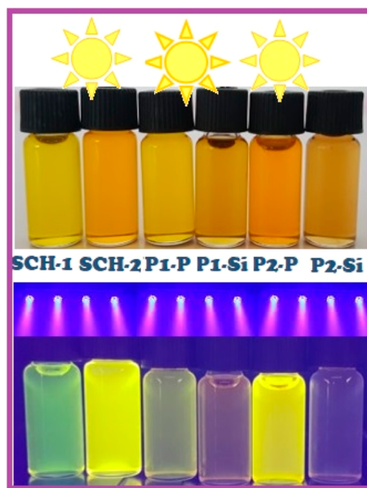
Figure 6. Photographs of SCH-1, SCH-2, and their respective P- and Si-oligo(azomethine)s under sunlight vs UV light (366 nm) in DMF.
