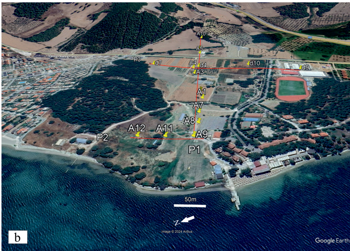
Figure 1- a) Geological setting of Biga peninsula (Okay and Satır, 2000) b) The study area and measurement stations for the DCR method (yellow pins).
